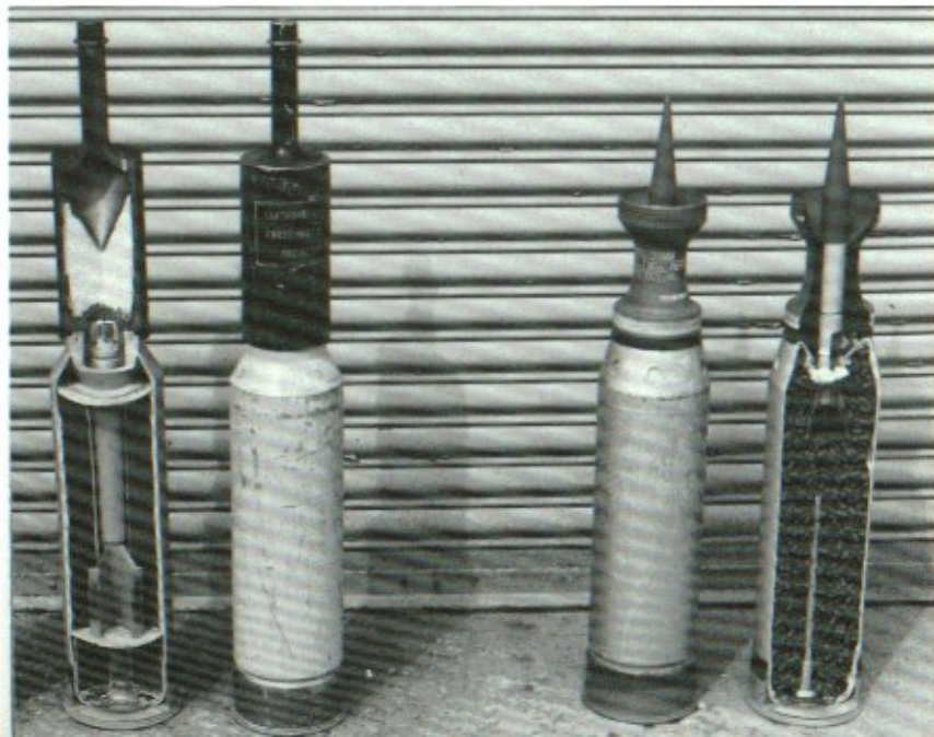
These shells and their cutaway counterparts are used for classroom instruction for M1 crews. The shell on the left is the M830 HEAT-T while the round on the right is the M865 TPFSDS-T. The M830 is a standard round carried on the M1 while the M865 is a training round. (Mesko)
