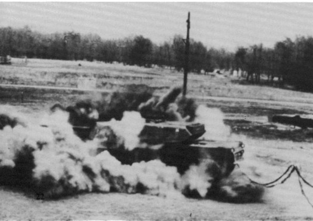
The M1 was subjected to a number of survivability tests with live ordnance to simulate actual battlefield conditions. In this test a captured Soviet mine is exploded under the hull. Test results showed that the M1 was one of the best protected vehicles in the world. (Green)
