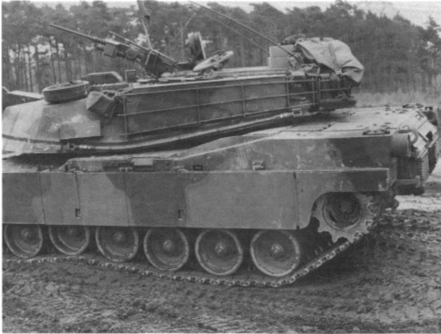
The twenty-five inch track retainer plate over the drive sprocket was deleted on the M1A1 and the rear armored side skirting was modified to help cut down on the buildup of mud and debris around the drive sprocket. (Jerchel)
