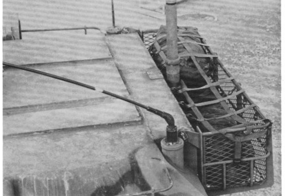
This early production IP M1 was modified in the field with a bustle rack which featured wire mesh to keep the crew's gear from falling out. The old style stowage straps were also used to keep gear from being bounced out of the basket when the tank ran over rough ground. (U.S. Army)
