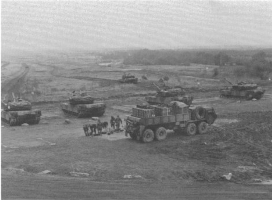
M1A1s on the firing range in Germany await instructions to move up to the firing line. The vehicle in the foreground is the new M977 Heavy Expanded Mobility Tactical Truck (HEMTT) which has the speed to keep up with the M1 and is far safer than the M520 GOER which had been used to resupply tank units in the field. (Jerchel)
