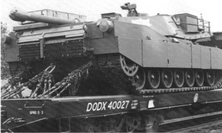
This early production M1 is securely chained down on a railway flat car for delivery to an Army unit. The gun barrel, sights, and all glass parts have been taped over to protect them during shipment. (Mesko)
