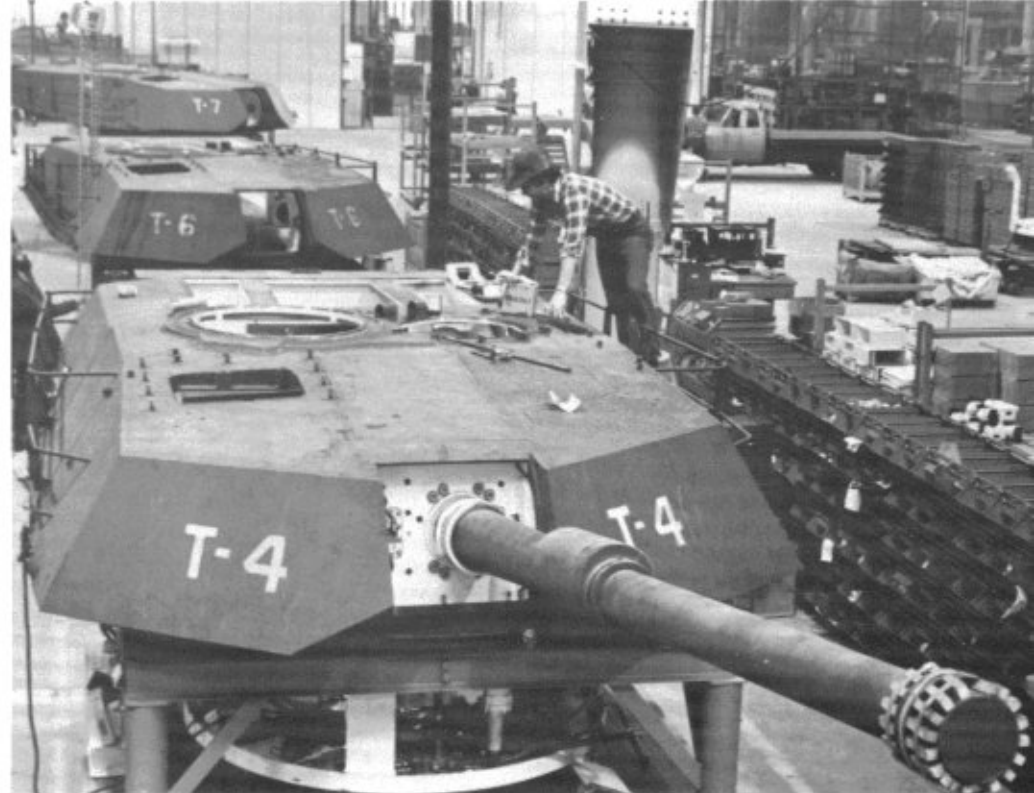
(Above) A nearly complete turret, fitted with the 105mm gun and turret basket, moves down the assembly line. The screws sticking up in front of the commander's station mark where the cover for the gunner's sight will be located and bolted down. (Wagner)
