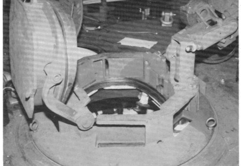
The commander's hatch can be pivoted to a horizontal position to provide overhead protection from shell bursts. In this way the tank commander can raise the hatch to get a clear view of the area yet remain protected from enemy fire. (Wagner)
