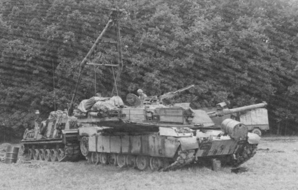
The Abrams has proven relatively trouble free in the field. When problems have occurred they have been handled quickly by repair crews. The crew of this M88 recovery vehicle helps pull the engine pack on Birth Control , an M1 from the 2nd Armored Division during exercise Certain Strike . (Jerchel)
