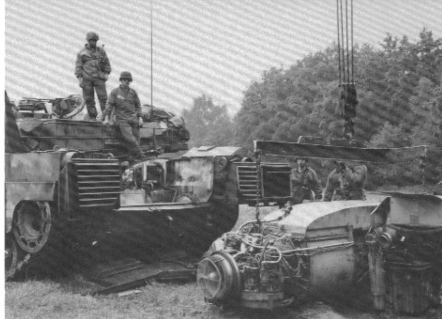
Changing a power pack on the Abrams can be done in the field in about an hour, enabling the tank to quickly return to action. This is a dramatic improvement compared to the four hours needed to replace an M60 engine. (Jerchel)
