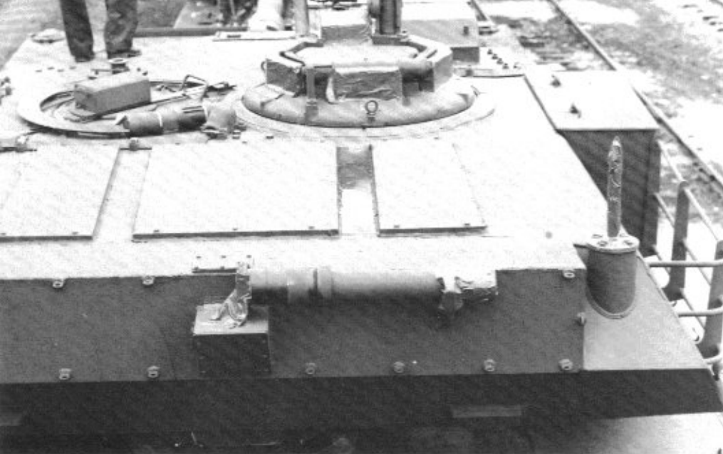
The M1 incorporated numerous features to increase survivability. The three large plates on the turret roof are blast panels which are designed to channel an ammunition explosion out through the roof in the event of a hit. The folded tube in the foreground is the windspeed/temperature sensor. (Mesko)
