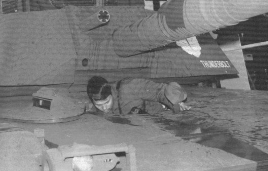
An M1 crewman enters the driver's hatch on the first production M1. Like the earlier M48 and M60 tanks, the M1's driver is located in the center of the hull with a hatch that is pushed up and swung away to gain access to the tank. (Wagner)
