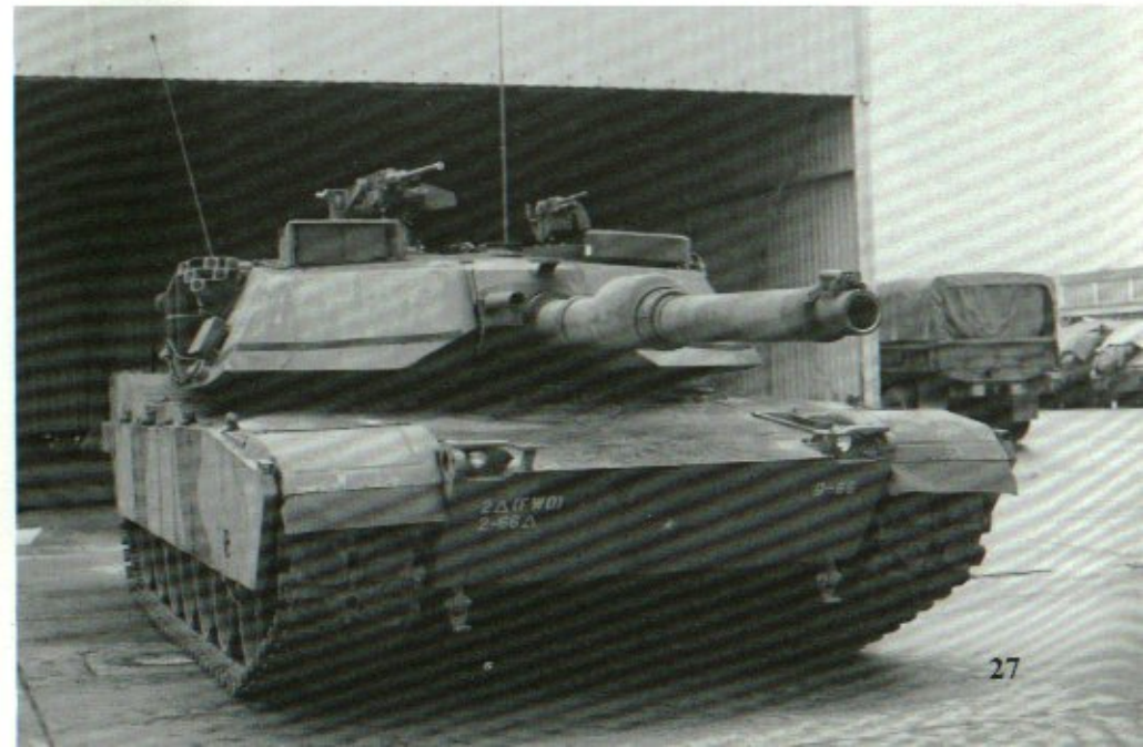
The headlight guards on the M1A1 differ from the M1 being flatter and slanted slightly forward. These revised guards also have a slight dip on the top and have only one attachment bolt. (Jerchel)
