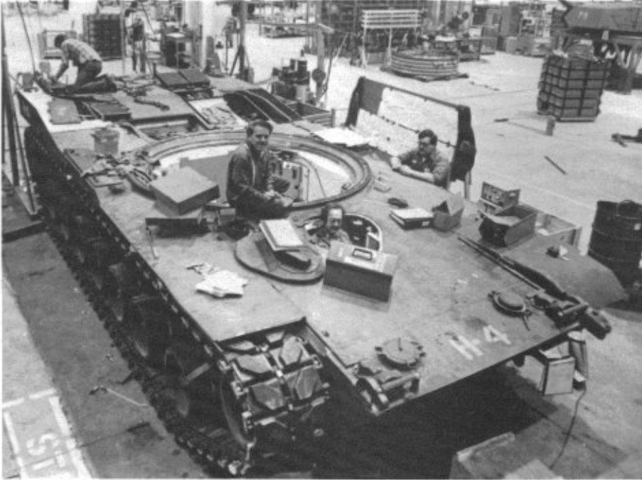
(Above) Workmen install equipment on a nearly completed M1 hull on the assembly line. The code H-4 on the hull is the factory identification code for the hull which will be mated with a turret with the same factory code during the final assembly process. (Wagner)
