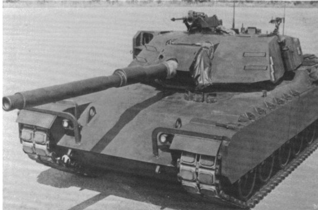
The General Motors XM1 prototype was powered by a conventional diesel engine. The vehicle was intended to offer the Army a modern, low silhouette vehicle with relatively few developmental risks and was favored by the Army. (Wagner)
