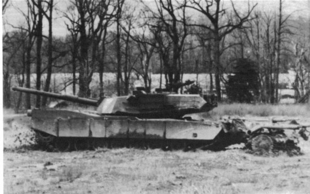
This M1 was fitted with a version of the mine roller installed on the M60 tank to determine if it could be modified for use on the M1. Aside from minor modifications needed to mount the roller to the M1 chassis, the standard kit worked well and is now being procured for use on the M1. (U.S. Army via Armor Magazine)
