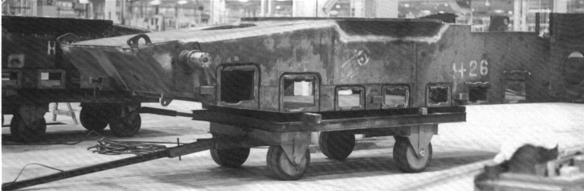
(Above) The hull of an M1 rests on a dolly ready to be moved to the assembly line. The large square openings in the sides of the hull are the attachment points for the bogie wheel assemblies. (Wagner)
