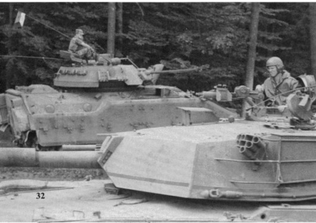
An M1 of the 1/64th Cavalry, 3rd Infantry Division (Mechanized) is parked alongside its Cavalry stablemate, the M3 Bradley. The Bradley was designed to give the infantry an armored personnel carrier which had an operating speed similar to that of the M1. (Green)
