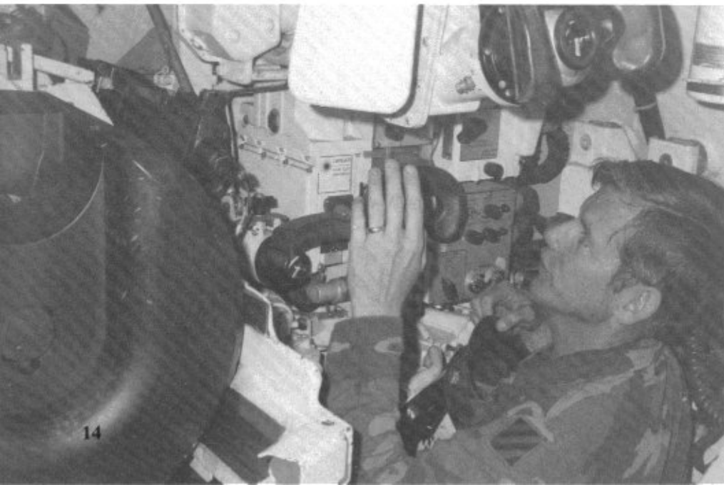
An M1 gunner mans his station inside the turret of the Abrams. His hand is on the gun sight, directly above his head is the tank commander's sight, while to his left is the breech for the M68A1 main gun. The coaxial machine gun is mounted just to the right of the main gun. (Green)
