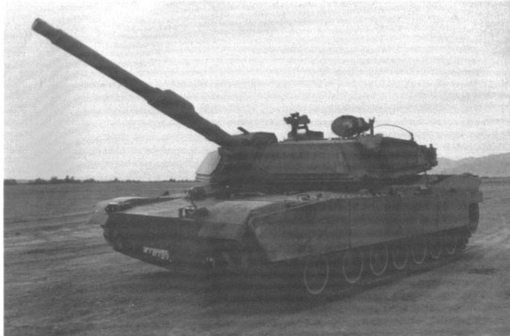
The most obvious change between the M1 and the M1E1 was the German manufactured 120MM main gun. Fourteen M1s were fitted with the new weapon during 1981 to test the gun/turret combination. (Green)
