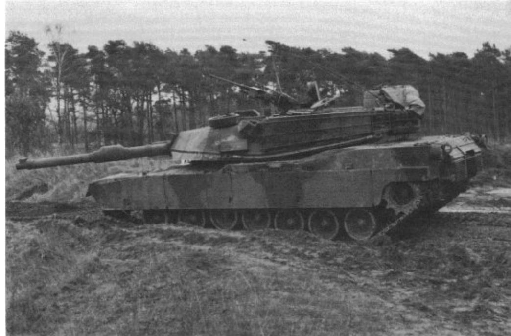
This M1 is moving along a dirt road up to its firing position on the practice range. The front suspension has shifted upward as the tank moves over the uneven road surface.
