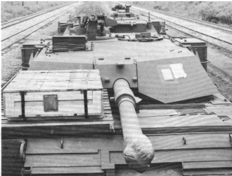
Additional equipment for the M1 is stored in the wooden box secured to the rear decking. Besides covering the gun barrel opening, the protective tape also covers the muzzle reference system to protect it from damage. (Mesko)
